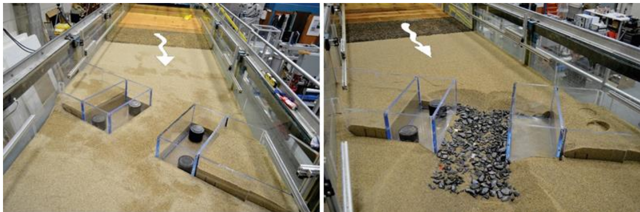
Figure 77. Photos. Comparison of run 11 as-built riprap installation (left) and at equilibrium scour (right).
