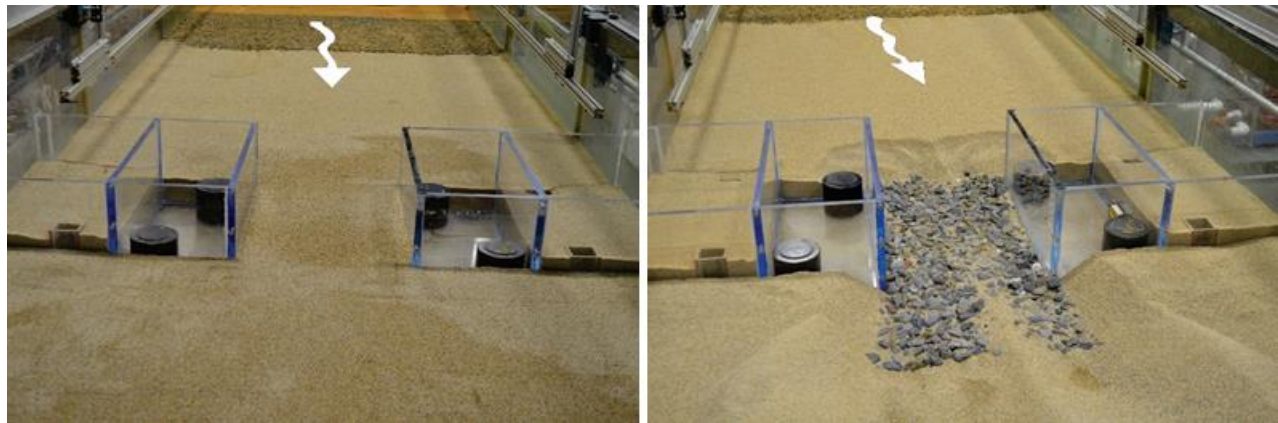
Figure 73. Photos. Comparison of run 8 as-built riprap installation (left) and at equilibrium scour (right).
