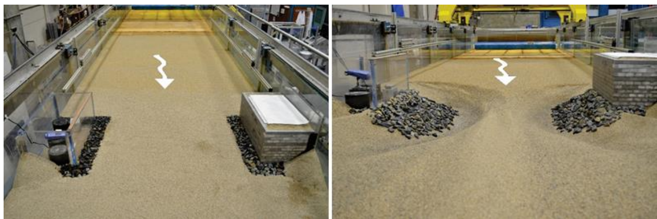
Figure 65. Photos. Comparison of run 3 as-built riprap installation (left) and at equilibrium scour (right).
