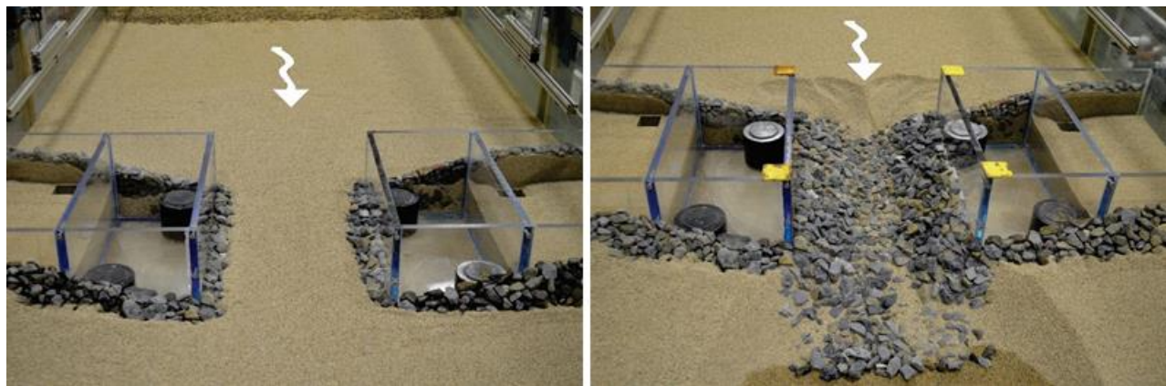
Figure 75. Photos. Comparison of run 9 as-built riprap installation (left) and at equilibrium scour (right).
