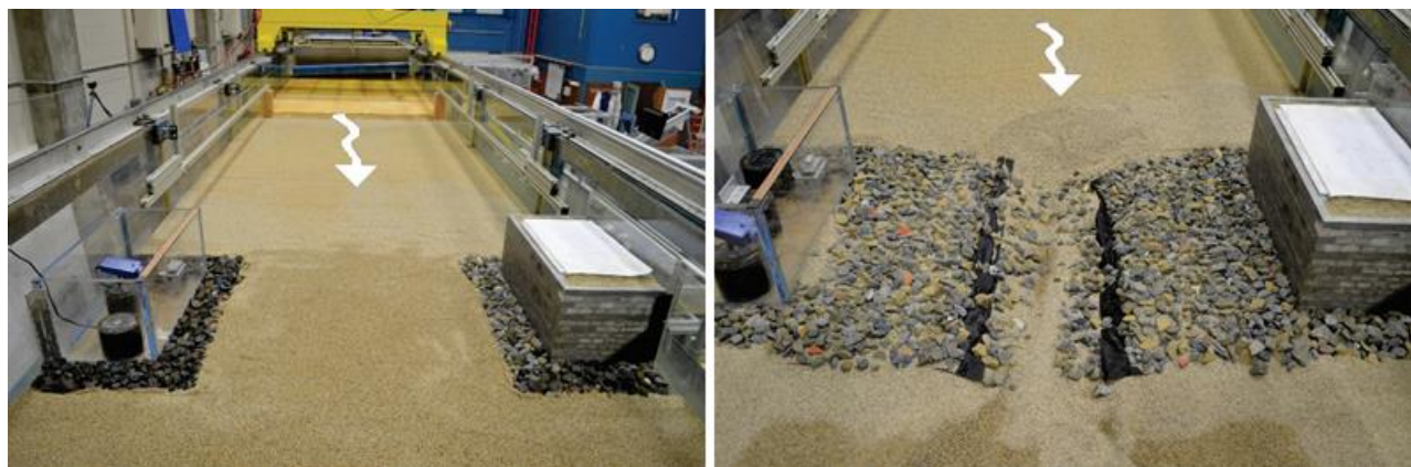
Figure 63. Photos. Comparison of run 2 as-built riprap installation (left) and at equilibrium scour (right).
